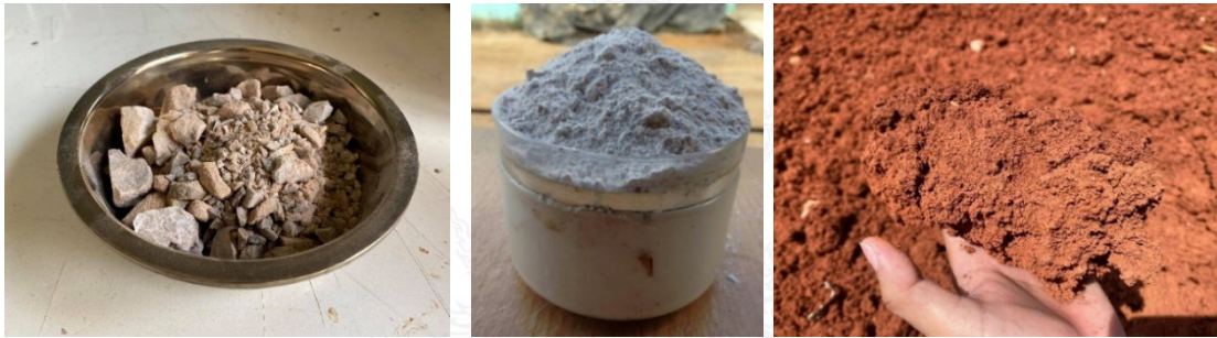
(a) Stone dust before crushing (b) Stone dust crushed (c) Laterite soil
