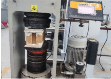
Fig. 4 Compressive strength test of interlocking block
