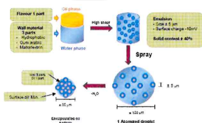
Figure 1. Proposed mechanism: Encapsulated flavour (generation by Dr. Werawat, 2009. Siam Modified Starch Co.,Ltd., SMS)
