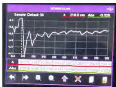
Figure 3.2 Display of spectrophotometer The channel marked in red is the wavelength range in nanometers (nm.). The green line is the ozone concentration in milligrams per milliliter (mg./ml.)
