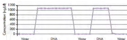
Figure 4: DNA carry over was analysed by measuring sample concentrations (via the in-built sample port), which were immediately followed by water.
