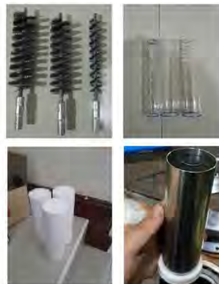
Figure 18 Assembly of a test kit for installation on stainless steel tubes and glass tubes inside, which together constitute the dielectric layer
