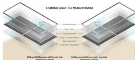
Fig. 3. The development of c-Si module technologies
