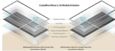
Fig. 3. The development of c-Si module technologies
