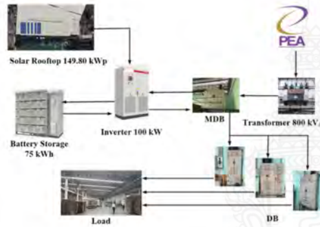
Fig. 9 Schematic diagram of hybrid solar rooftop 149.8 kWp.
