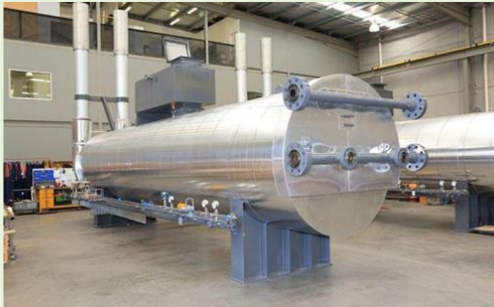
Water bath heaters
