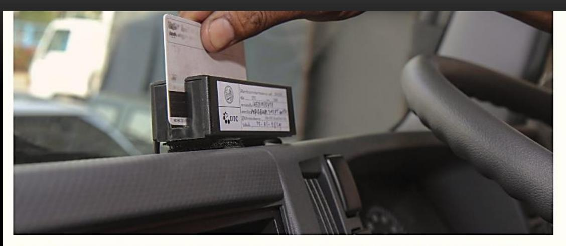
A driver of a public vehicle is required to swipe a card through a GPS-linked reader, to selfverify his identify before driving.
